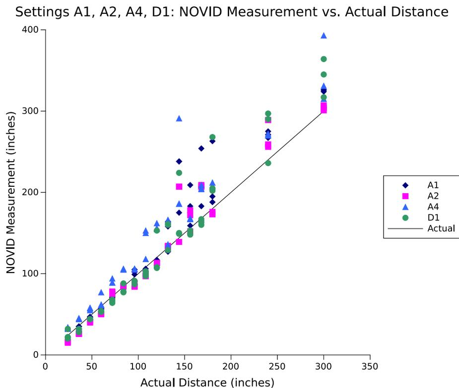
Figure 2: All distance measurements for Settings A1, A2, A4, and D1. Note that the region of highest accuracy extends up to 108 inches (9 feet), while measurements consistently provide upper-bounds on the actual distance.
